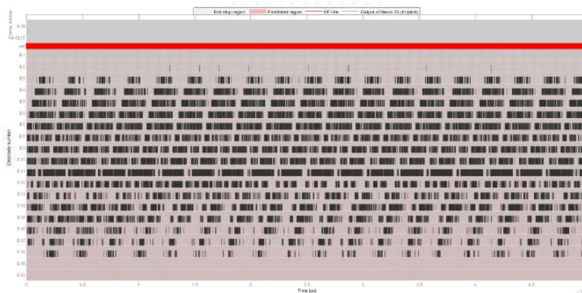
Figure 27: Example of former EDG used to our analysis, (the electrodes being numerated from apex to base of the cochlea, first number correspond to low frequency and last to high ones, so it's upside done compared to spectrogram classic plots, thanks to Dr.Rafael Attili Chiea code, we could superposed EDG and spectrogram.
