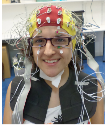
Figure A.1: Biosemi system using 64 electrodes placed according to the modified 10-20 system, together with 8 additional electrodes placed on the mastoids and circumocular positions.
