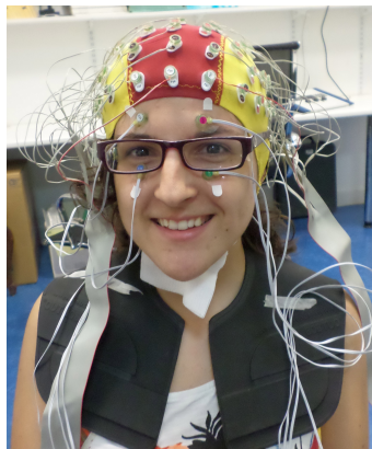
Figure 2.4: Biosemi system using 64 electrodes placed according to the modified 10-20 system, together with 8 additional electrodes placed on the mastoids and circumocular positions.
