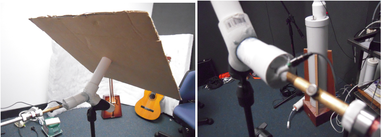
Fig 2.4: Experimental device for the measurement of the impedance at the “glottis”.
